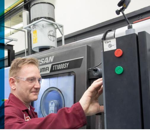
The **F Monitor Essential** measures velocity pressure to check the airflow is correct and a simple traffic light system makes it easy for the machine operator to identify any potential issues.
